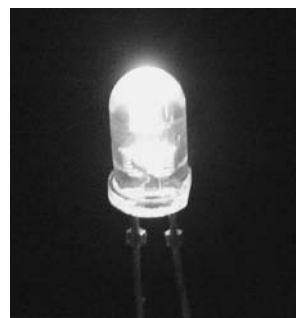
Figure 5. The photograph of \text{LiBa}_{0.95}\text{PO}_4:\text{Eu}^{2+}_{0.05} -InGaN LED under 20-mA current excitation.
